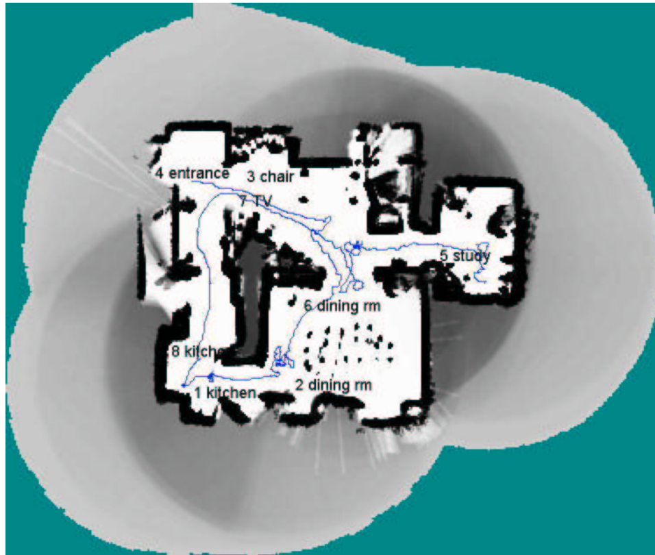
Figure 6.5: Laser range finding data from the ground floor of a house: Dark regions correspond to obstacles like walls and furniture, white regions correspond to free space. Once a map has been learned, any new obstacles which are not in the map are assumed to be people. In this way, the trajectory of a moving person (shown as a wiggly blue line) can be inferred. Various places where the person likes to spend a lot of time are labelled, and are considered landmarks or goals. This data is from [BBT02].
